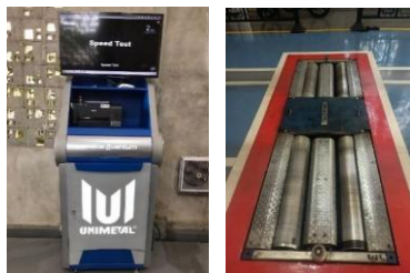
Gambar 2. Alat Uji Speedometer
