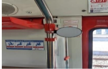
Gambar 3. Alat Receiver Tiang Prioritas
